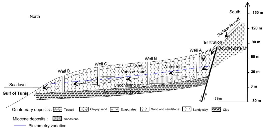
Fig. 3. Hydrogeological cross section of the Grombalia aquifer (Ben Moussa et al., 2010).
