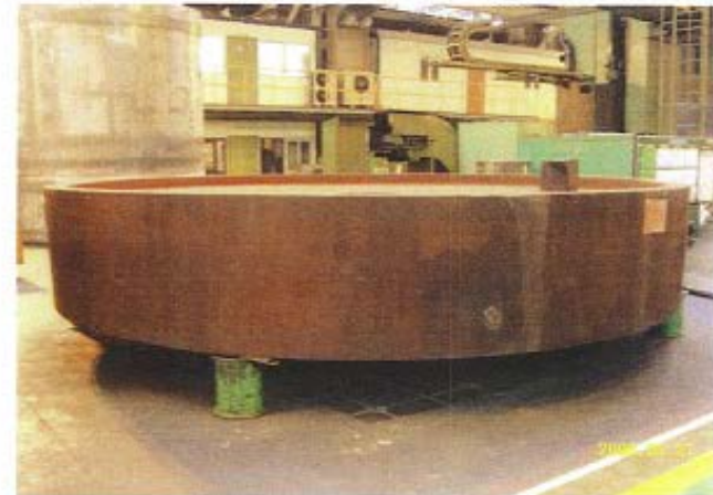
#4B : QHT of Forging Material has been completed.
