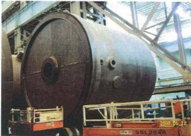
#3A : Tubesheet Drilling has been complete.
