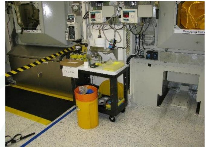
Packaging cell where contamination event occurred, with radiation monitoring station subsequently installed as a corrective action
