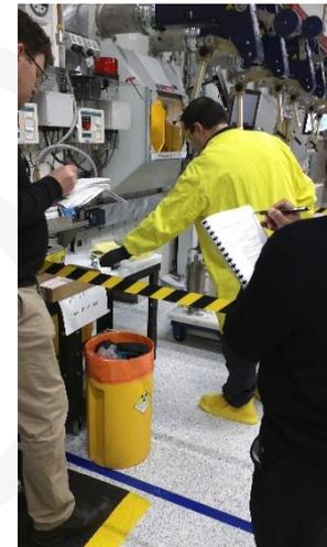
Contamination monitoring introduced after the event at the new Mo-99 production facility
