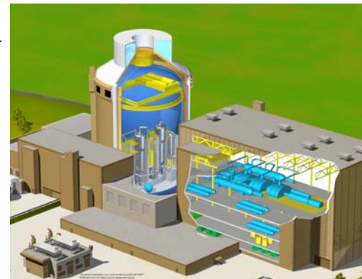
Cutaway view of the Westinghouse AP1000 reactor
