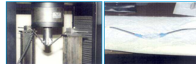
1987 bending test on PWR fresh fuel pins
