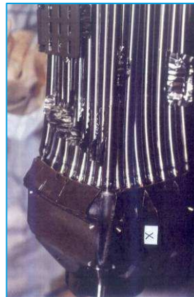
BWR 8x8 fresh fuel assembly loaded in the FS 74 cask
