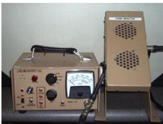
**Figure 7c.** Monitor for checking contamination of hands.
